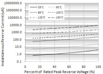
Figure 4. Typical Reverse Characteristics
