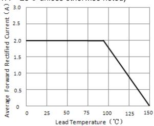
Figure 1. Forward Current Derating Curve
