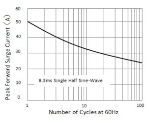
Figure 2.Maximum Non-Repetitive Peak Forward Surge Current
