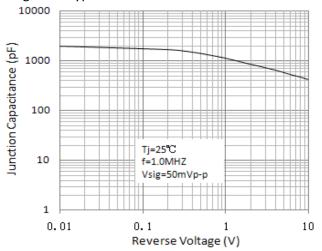
Figure 5. Typical Junction Capacitance
