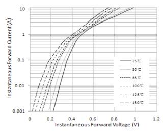
Figure 3. Typical Instantaneous Forward Characteristics
